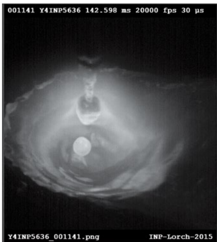
Fig. 1: The primary droplet forms at the end of the wire.
